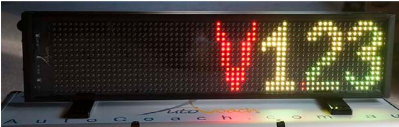
*Velocity reading on ACS250 using SmartWatch in “Speed” mode showing 1.23 meters per second split.*
