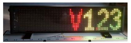
Velocity reading on ACS250 using SmartWatch in "Speed" mode showing 1.23 meters per second split.
